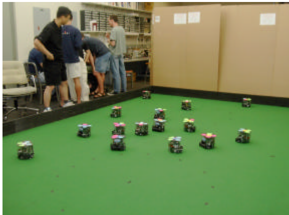
Figure 1: Photo of the actual RoboFlag test-bed.
